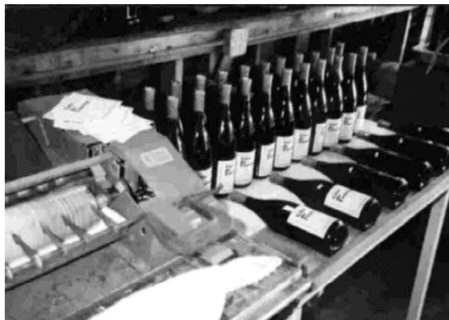
Figure 4. Label pasters, like the one on the left, apply glue to plain paper labels quickly and easily.
